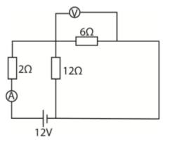
In the circuit above, the battery has negligible internal resistance. Find the ammeter and voltmeter readings (4marks)
