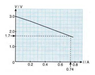
From the graph, determine the e.m.f. of the cell and its internal resistance.
